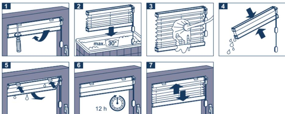
**1** Remove the blind. **2** Wash the blind using a mild detergent solution and water at approx 30°C. **3** Rinse thoroughly. **4** Fold the fabric parcel together and squeeze the water out by pressing the rails of the blind together until the blind is no longer dripping wet. **5** Hang the damp blind. **6** Leave it closed to dry. **7** Open and close the blind several times during the drying process to prevent the pleats from sticking together.
